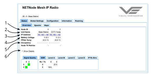
This displays detailed status information of received signal quality and enables navigation between nodes. The Status tab is divided into three sub-tabs:
