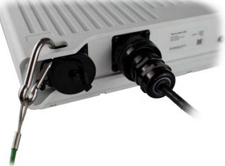
The hanging strain relief cable should be connected by clipping the carabiner to the slot in the ODU, as shown here.
