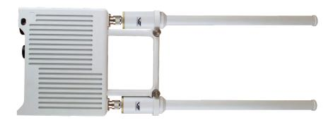
Now connect the weatherproof end of the 20m interface cable to the "Primary' amphenol connector on the ODU, as shown below.
