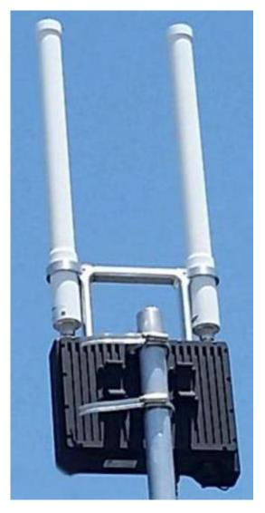
Note: When handling the ODU the user should be careful to avoid manoeuvring the unit by handling the antennas. Doing this can cause damage to the antenna connectors.
