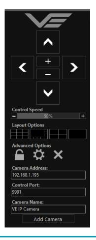
Selecting the right hand side icon allows the user to manually add a camera by IP address.
