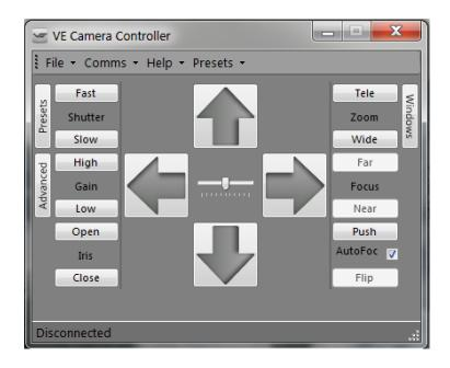
It is necessary to connect a USB to serial comms lead to the PC. The operating system of the computer will allocate this a COM port number.
