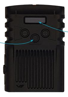
The OLED screen gives battery % remaining and the time to expiry in minutes.
