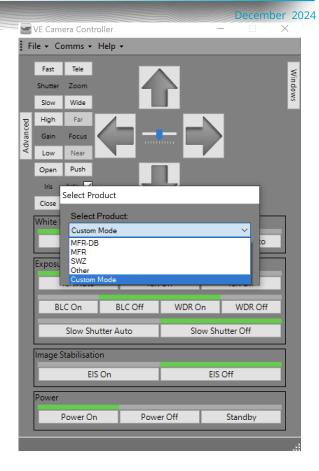
Since the MFR-DB does not support a TCP/IP connection only RS232 communications are supported.
